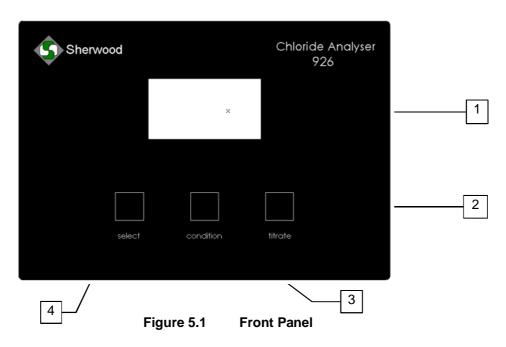
1. Display screen, 2. 'titrate' button, 3. 'condition' button, 4. 'select' Units button.
