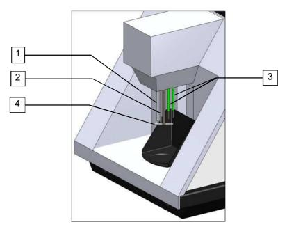
Figure 8.1 Electrodes and Electrode Head
