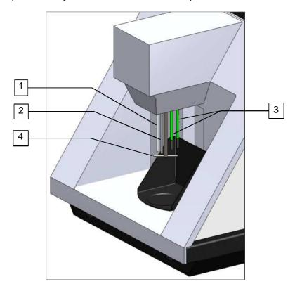
Figure 2.1 Electrode Head
